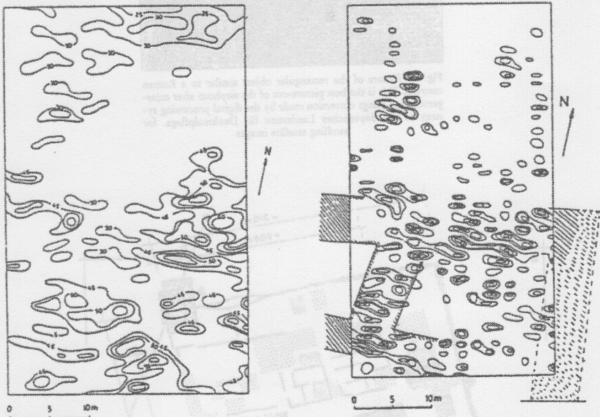
Fig. 5. Resistivity maps. A: apparent resistivity map constructed from measurements with dipole-dipole array with a dipole distance of 3 m; B: filtered map of A, applying a symmetrical edge filter in NW-SE direction and of \odot sum. The interpreted linear feature is hatched
